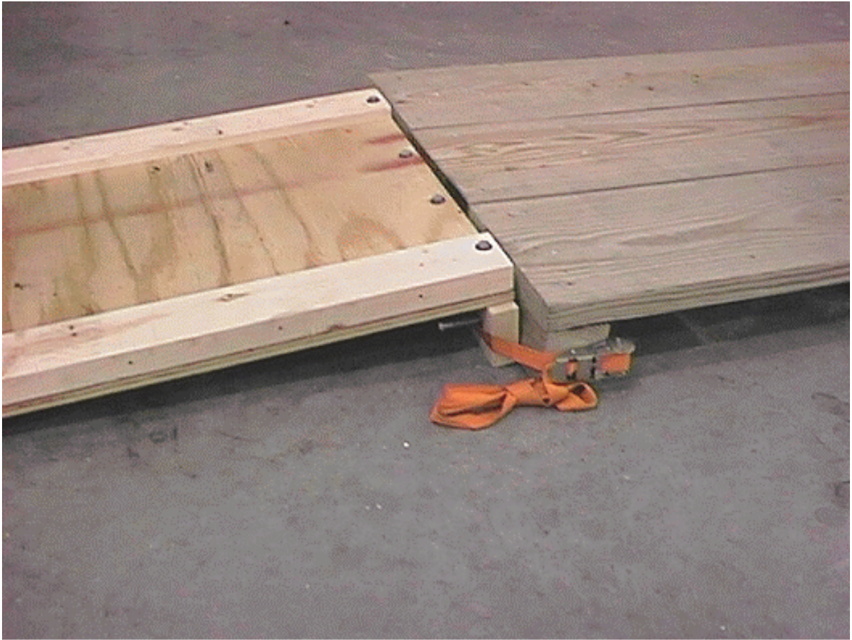
Figure 3: Set the RAMP up against the end of the crate base and secure it to the base 4x4 with one of the tie down straps from the maser.
